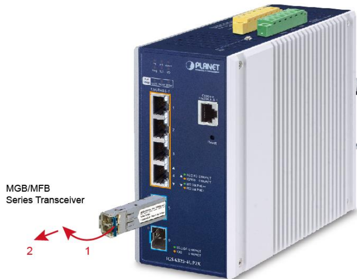
Figure 2-3-2: Pull out the SFP/SFP+ Transceiver Module
