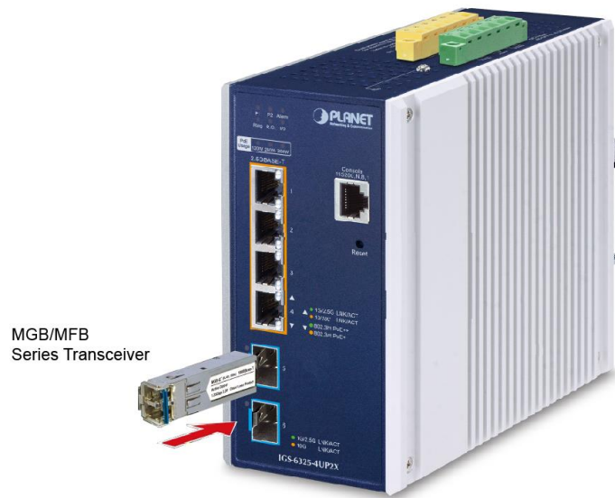
Figure 2-3-1: Plug in the SFP/SFP+ Transceiver
